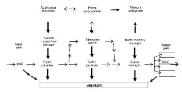
FJRE-Flexible Intelligent Routing Engine
